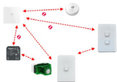
Zigbee Mesh network example
