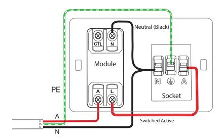
Circuit looped, single switched socket wired downstream of the timer
