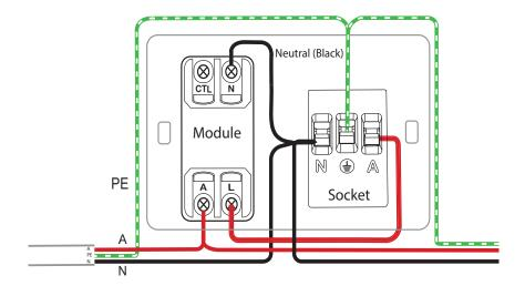
Note: Loop out of the Active terminal "A" of the module, as shown in the diagram. Do not loop out from the Socket Active terminal "A".
